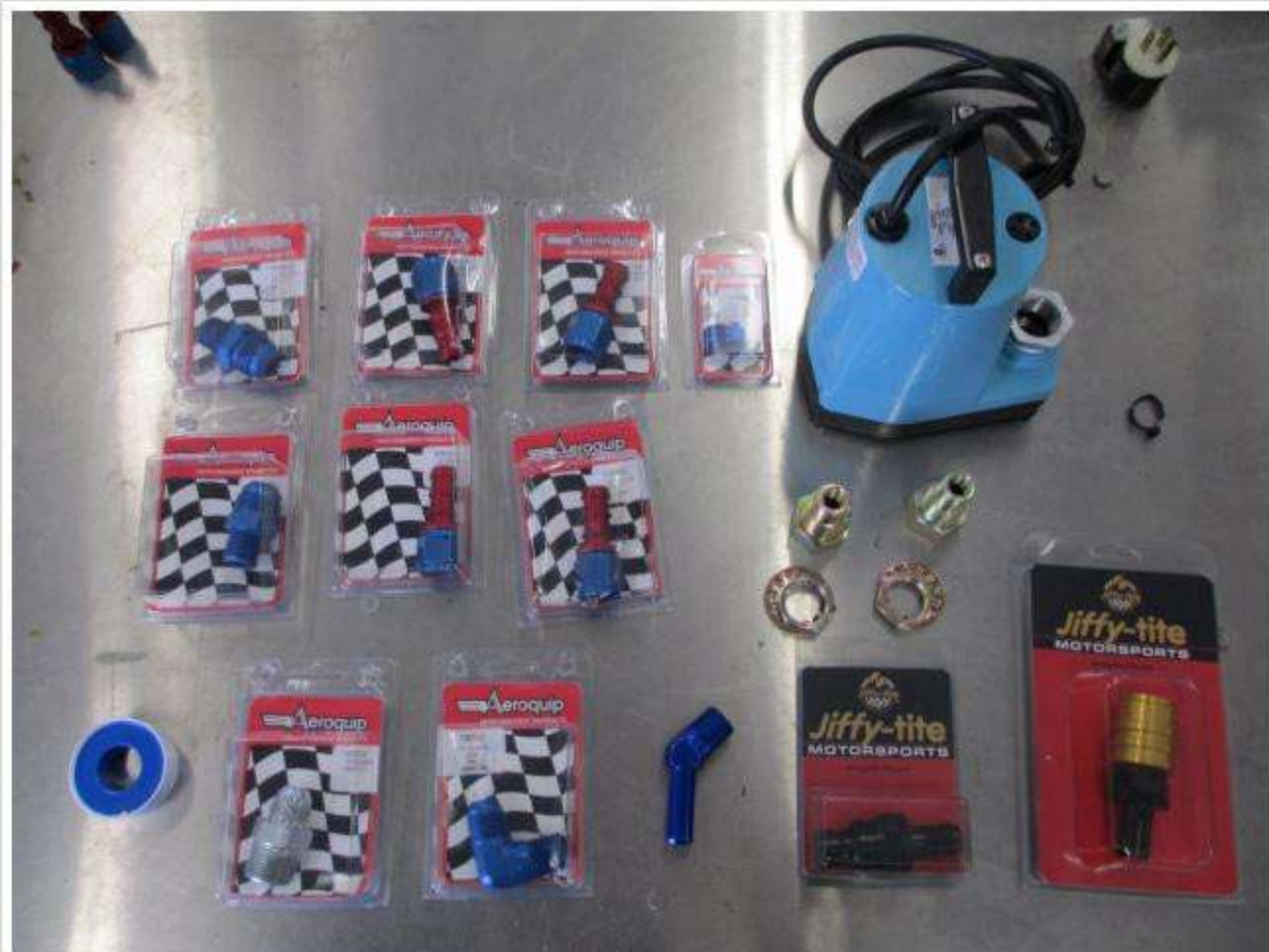
Some of the components used to create the Chiller including the 110V submersible pump seen at top right.
